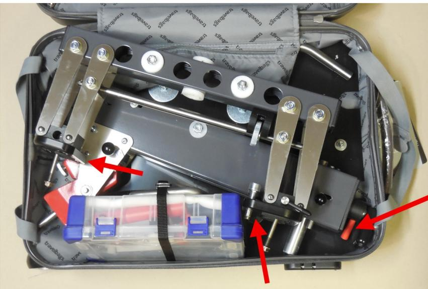
To create maximum support of the turntable make sure that it is supported on the edge of the bracket of the tensioner and on the round support shown by the arrows on the picture. Create this situation as follows.
